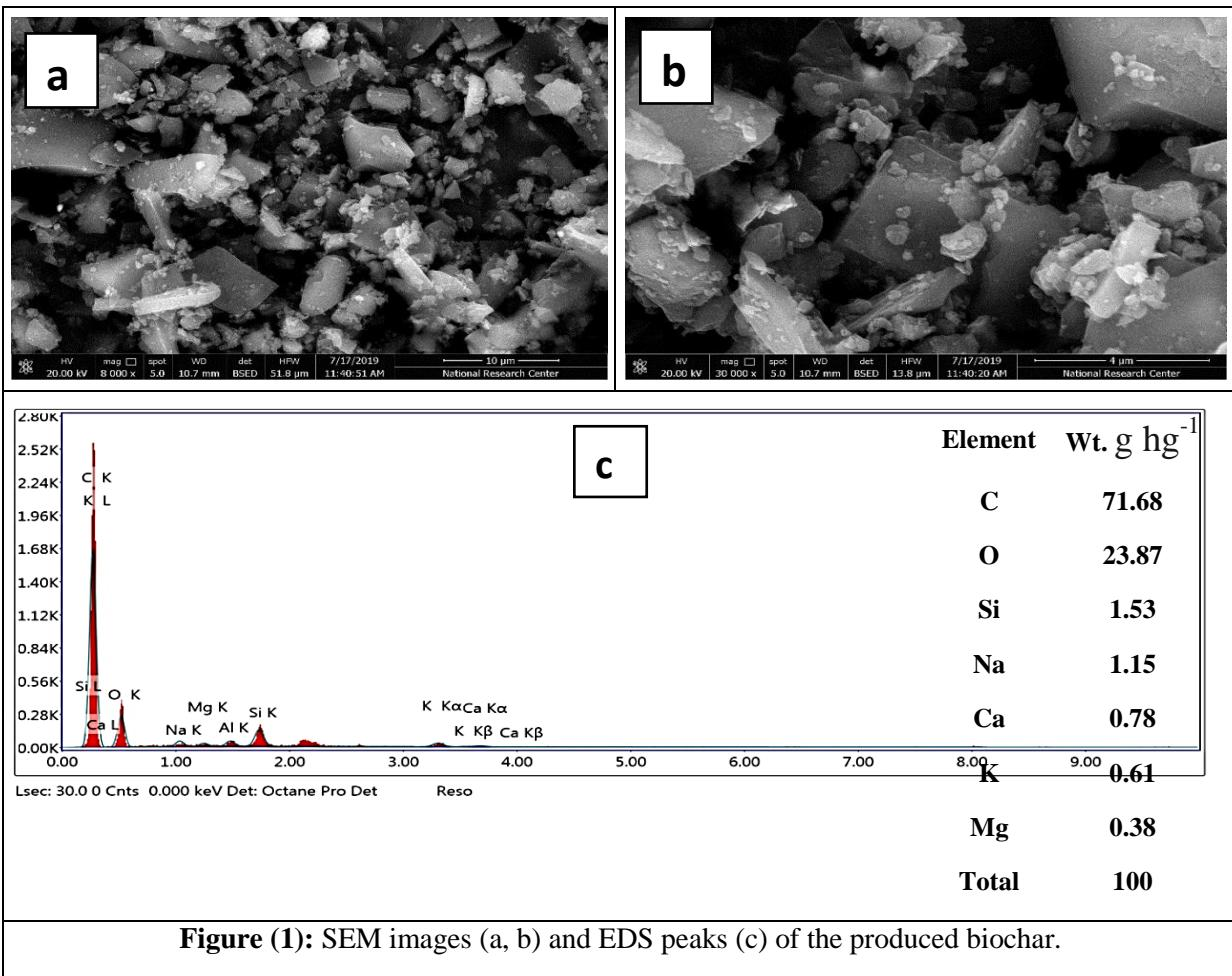
**Figure (1):** SEM images (a, b) and EDS peaks (c) of the produced biochar.
